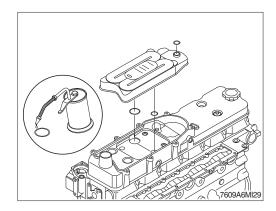
(10) Install the crankcase breather filter cover. Install the filter cover capscrews.
