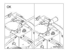
During filling, air must be vented from the engine coolant passages.
