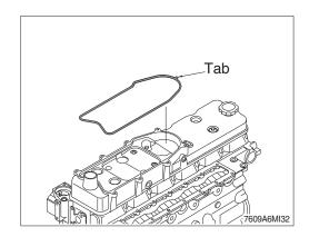
(8) If the gasket was removed, install the gasket into the rocker lever cover groove starting with the tab end first. Then install the corners opposite the gasket tab end. Finish by pushing in the sides (see illustration).
