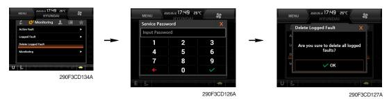
• The logged faults of the MCU, engine ECM, air conditioner or AAVM (option) can be deleted by this menu.
