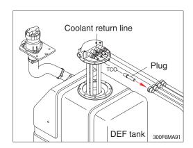
(3) Rotate the DEF/AdBlue® level sender counter-clockwise about 20 degree with the Jig (P/no: HDB030-0001).
