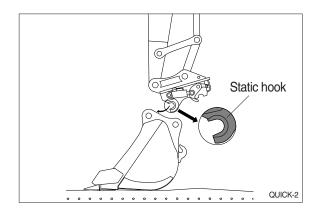
(4) Operate RCV lever to bucket-in position.
