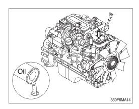
(10) Operate the engine at low idle and inspect for leaks at the filters and the drain plug. Shut the engine off and check the oil level with the dipstick. Allow 15 minutes for oil to drain down before checking.
