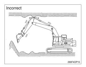
10) Do not use the dropping force of the work equipment for digging.
