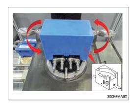
(4) Remove the DEF/AdBlue® level sender without removal of the plunger ring.
