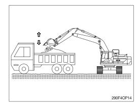
8) Operate stop of swing considering the swing slip distance is created by inertia after neutralizing the swing lever.
