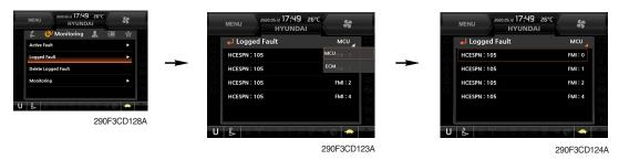
• The logged faults of the MCU, engine ECM, air conditioner or AAVM (option) can be checked by this menu.
