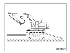
(2) Place the swing lock/fine switch to the LOCK position (if equipped) after the swing the machine 180 degree.
