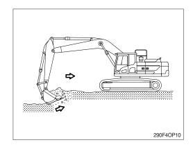
2) When lowering and raising the boom operate softly for the beginning and the end.In particularly, sudden stops while lowering the boom may cause damage to the machine.
