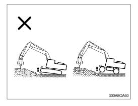
Do not extend the bucket cylinder fully and thrusting to raise the machine off the ground.
