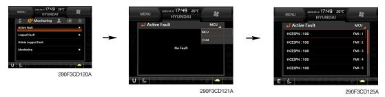
· The active faults of the MCU, engine ECM, air conditioner or AAVM (option) can be checked by this menu.
