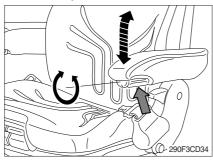
① The inclination of the armrests can be modified by turning the adjustment knob (arrow).
