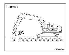
11) Do not use the bucket to crack hard objects like concrete or rocks.
